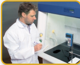
Face velocity measurement test
